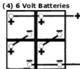
These are two of the most standard 12vdc battery installations. To the left there is a series-parallel battery. To the right is a standard 12v parallel hook up.
