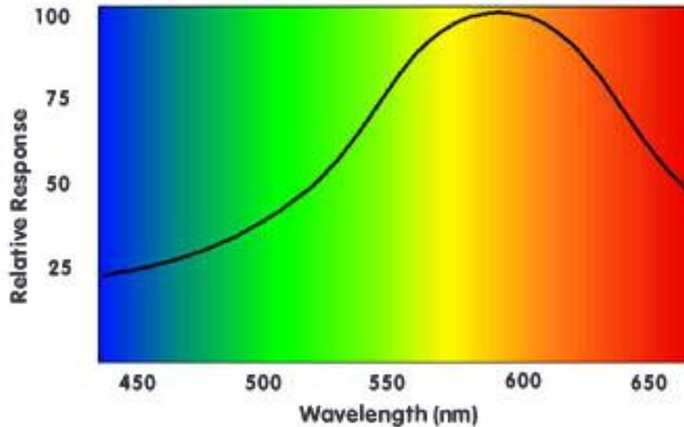
Peak wavelength is a function of the LED chip material. Although process variations are  $\pm 10$  NM, the 565 to 600 NM wavelength spectral region is where the sensitivity level of the human eye is highest. Therefore, it is easier to perceive color variations in yellow and amber LEDs than other colors.
