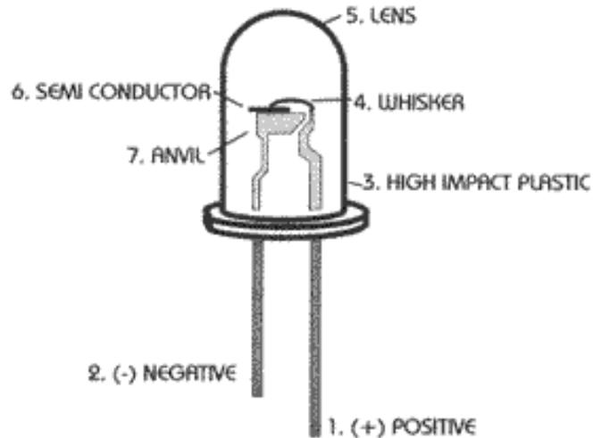
As you can see, the entire unit is totally embedded in epoxy. This is what make LEDs virtually indestructible. There are no loose or moving parts within the solid epoxy enclosure.
