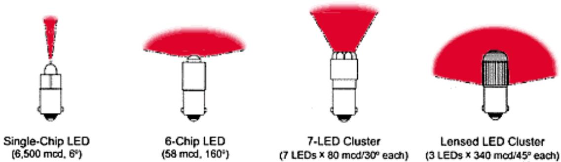
In each case, the amount of visible light depends on how the LED is being viewed. The single chip may be appropriate for direct viewing in competition with high ambient light. The 6-chip may be better suited to backlight a switch or small legend, while the cluster or lensed LED may be best to illuminate a pilot light or larger lens.
