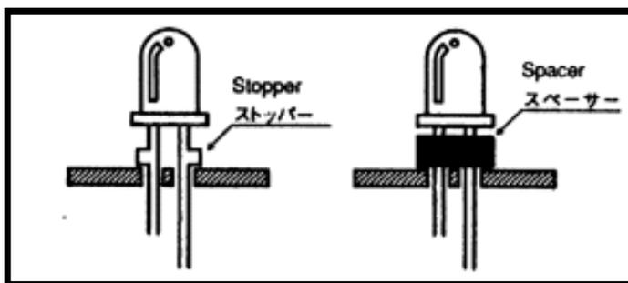
Use LEDs with stoppers or resin spacer to accurately position the LEDs. The epoxy resin base should not be touching the PC board when mounting the LEDs. Mechanical stress to the resin may be caused by the warping of the PC board when soldering.
