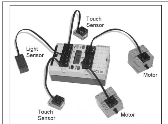
Figure 3. The RCX controller, motors, and sensors.
