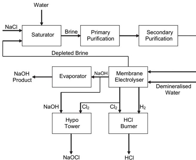
Fig. 7. Process flow diagram for chlor-alkali plant (Case Study 2).
