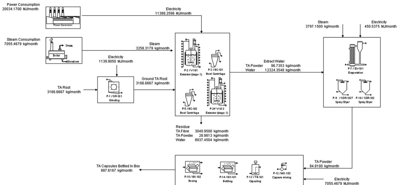
Fig. 5. Sectional electricity and steam input for Case Study 1 (Kuan, 2005).
