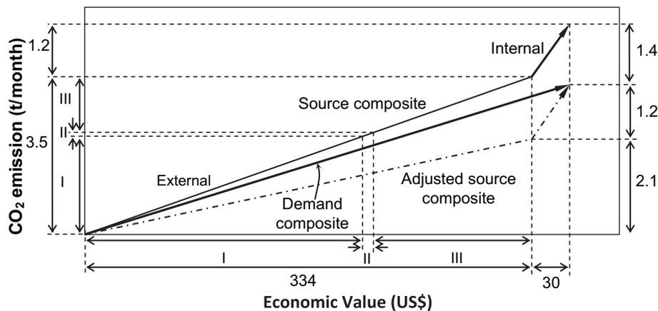
**Fig. 6.** Energy-based footprint composite curves for Case Study 1 (I: extraction, II: drying, III: packaging).
