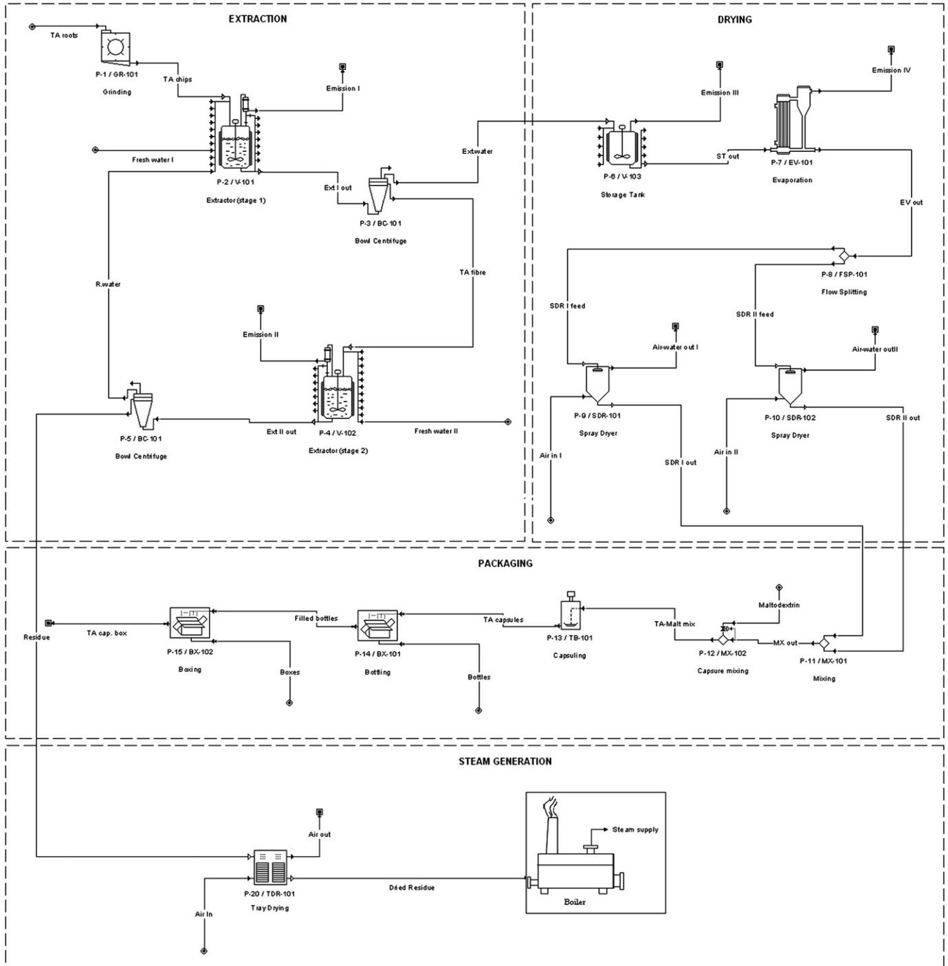
Fig. 3. Process flow diagram for TA extract production (Case Study 1).
